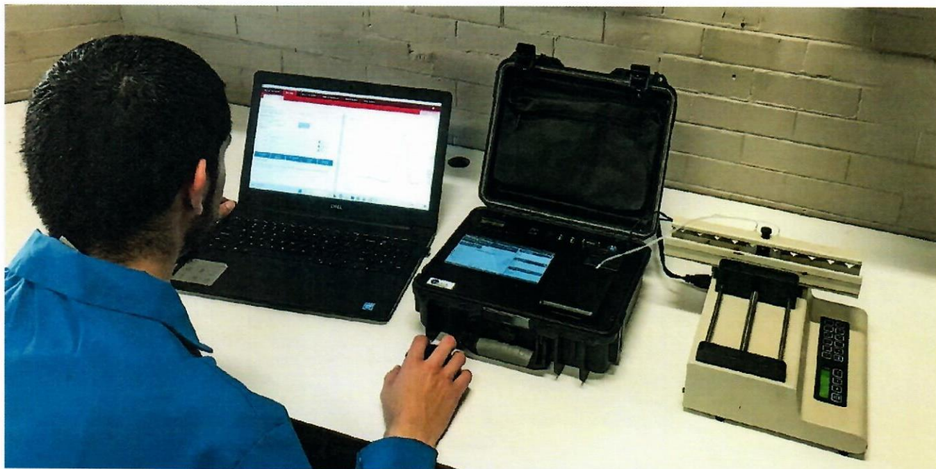
A technician tests a field-portable electrochemical per- and polyfluoroalkyl substances analyzer being developed by 2Witech Solutions.
